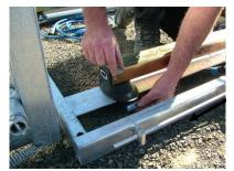
Using bolts with square washers, clamp the load bars to the Weigh Frame with the ridge of the square washer facing outwards. Put on flat washer, spring washer, and nut loosely until checked for squareness and tighten bolts using 18mm and 19mm ring spanner. These load bars can now stay permanently on the Weigh Frame.
