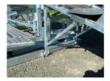
Put ramps stands in place and secure with rod.
