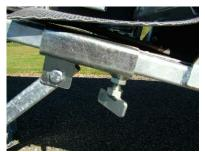
Place draft block under the front of the Draft before positioning Draft on ramp stand and lock into position.
