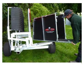
Using wheel as a pivot point, put the race onto the handler. Make sure the wall brace is in place under the anti-jump rails at the hinge end of race.
