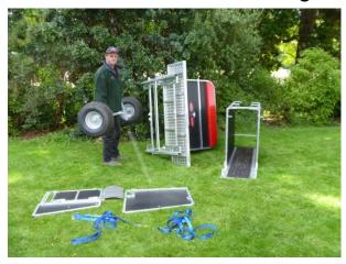
Remove gates from race. Place wheels in lugs. Long side of axle goes on pressure plate side.
