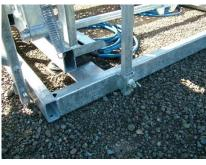
**Shifting:** To shift handler without Weigh Gear undo top load bar bolts and slide the handler off the load bars.
