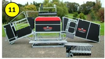
Place the access ramp over the base frame. Replace the gates on the approach race and move either, just the far, or both anti-jump rails forward. Test all gates to make sure
