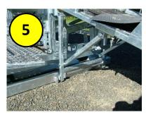
Put the ramp stands in place and secure them with pins and rubber rings found on the base frame.
