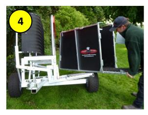
Using the wheel as a pivot point, put the race onto the handler. Make sure the wall brace is in place under the anti-jump rails at the hinge end of the race
