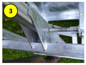
Pin the drawbar to the axle. Pull trailer down onto its wheels
