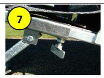
Lock into position by stretching the hand outwards to fit over the race floor. Tighten wing nut firmly
