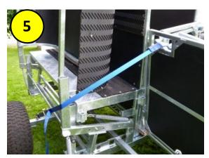
Replace gates and put the tie-downs in place. The front strap goes through the gate handle and ratchet handles at the rear of the handler
