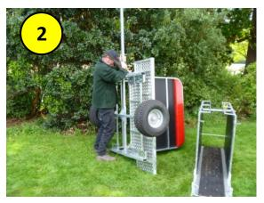
Feed the drawbar down through the holes, while holding the axle in place with your knee if needed.
