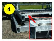
Roll the handler on top of the load bars until the slots on the handler line up with the holes on the top of the load bars. Put bolts in loosely so that you can still slide the handler to line up with the ramp stands
