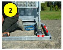
Centre the load bars on the base frame, with the cables facing inwards
