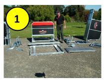
Set handler up in position. Roll handler over onto its back and position Weigh Frame against the base of the handler, so the Gadget Holder lugs are facing the rear.
