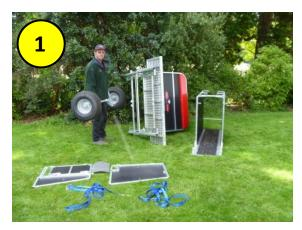
Remove the gates from the approach race. Place the wheels in the lugs, with the long side of the axle going on the pressure plate side
